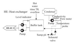
**Fig.4.** The improvement of control method for wastewater qualities.
