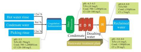
Fig.2. The process of wastewater reclamation and reuse in EGL.
