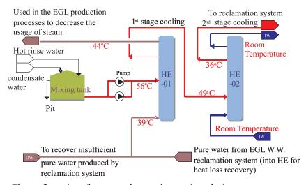
Fig.6. The configuration of two-stage heat exchanger for reducing wastewater temperature.
