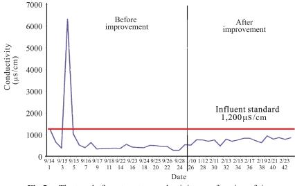
Fig.5. The trend of wastewater conductivity as a function of time.
